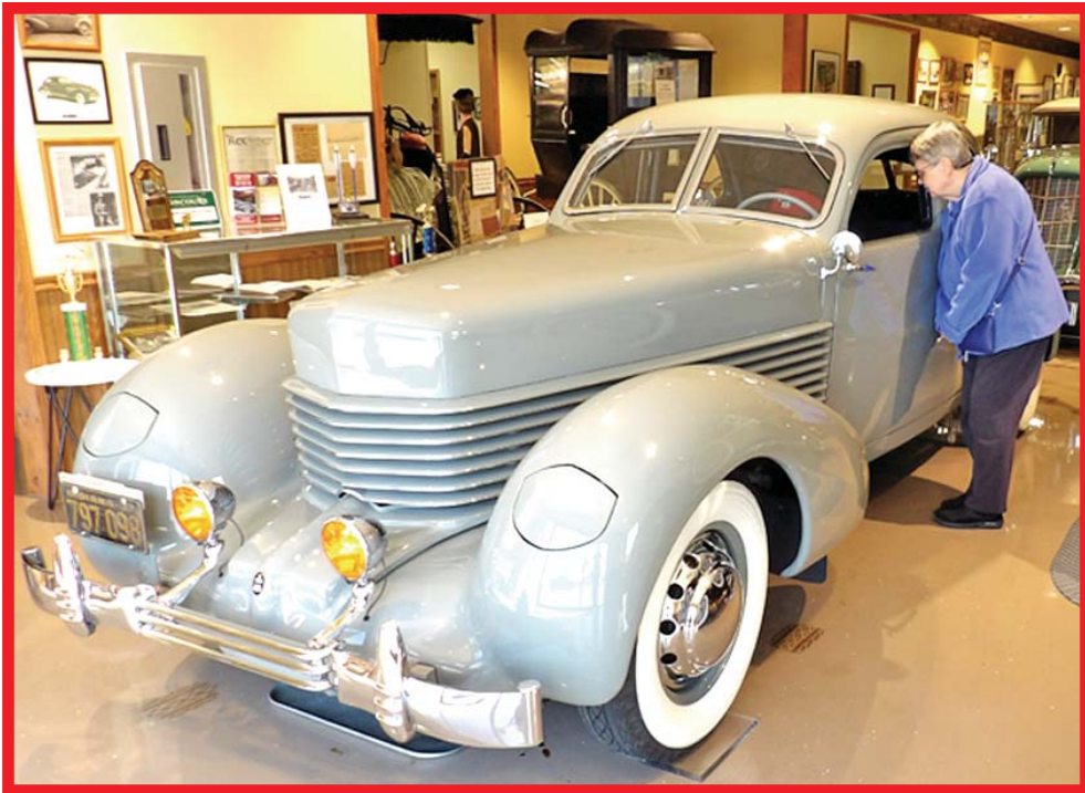
Sherry Dickerson, author's wife, checking out the beautiful interior of the 1937 Cord Beverly. This car has many innovative features, including front wheel drive, hidden headlights, and electric self starter.
