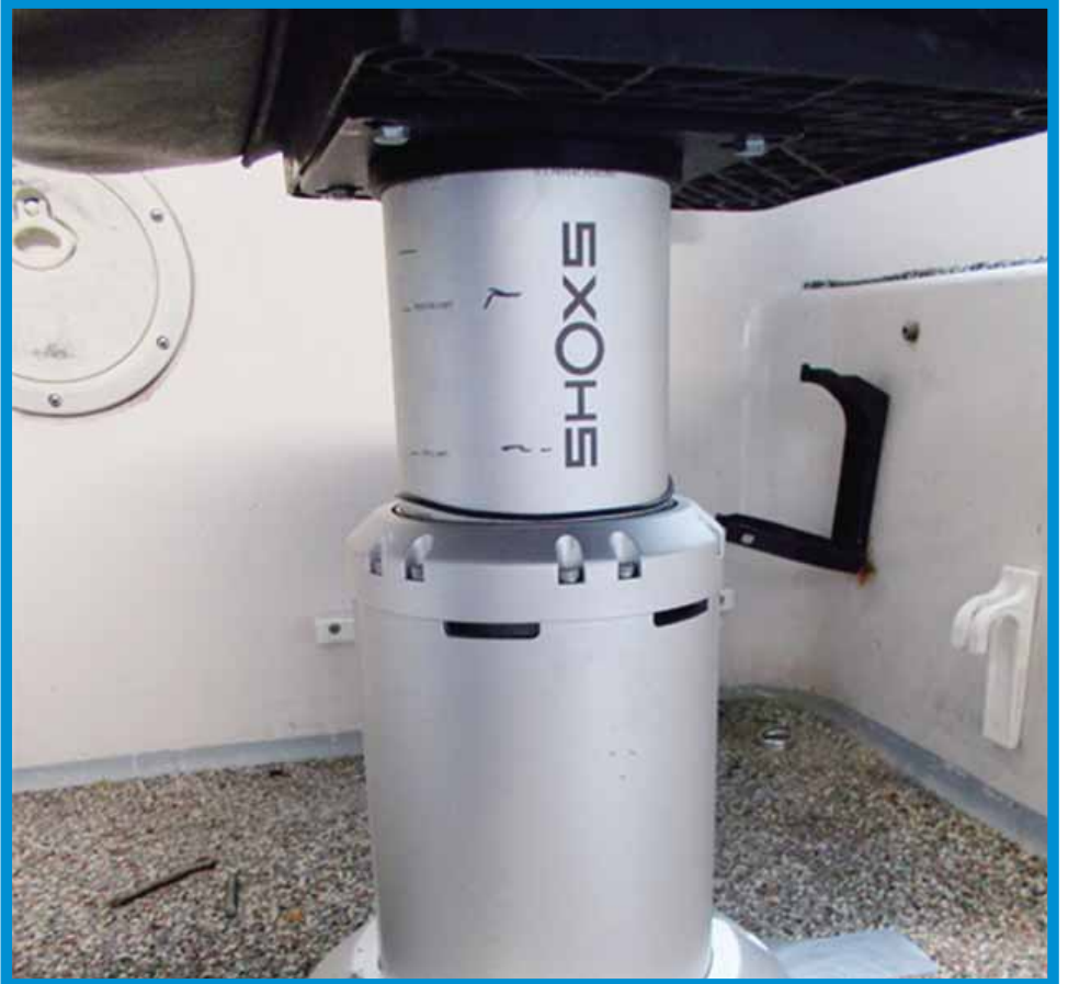
Installing a Shox, shock absorbing seat pedestal will save wear and tear on your back and smooth your boat's ride in bumpy conditions. (Author Photo)
