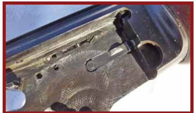
The ejector in its locked down position for cleaning the bore from the breech. Note that the lock screw slot is not aligned with the ejector. (Author Photo)
