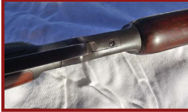
This is the Finger lever spring screw. There is no need to remove this screw. (Author Photo)
