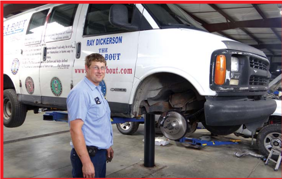
Joe Schirmer got right to work and found that both of my front brakes were bad. The noise I heard was the metal on metal contact when I was braking. (Photo by Ray Dickerson)
