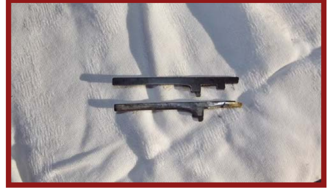
Firing pin on bottom is brass tipped and badly made. Firing pin on top is the correct firing pin. (Author Photo)
