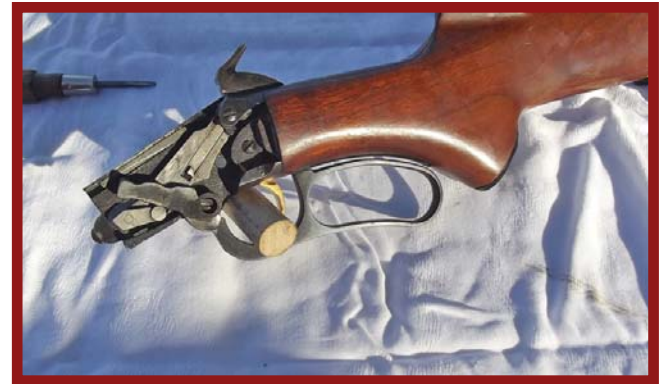
The Finger lever in the correct closed position and holding the bolt fully closed. (Author Photo)
