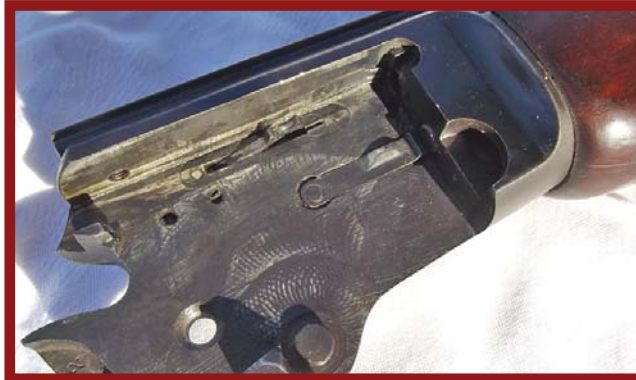
The ejector in its normal unlocked position. Note that the lock screw is aligned with the ejector. (Author Photo)
