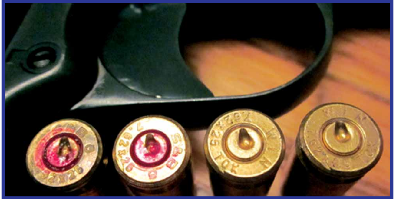
Firing pin wipe is indicated here. Note how the firing pin imprint is elongated probably due to early unlocking. (Author Photo)
