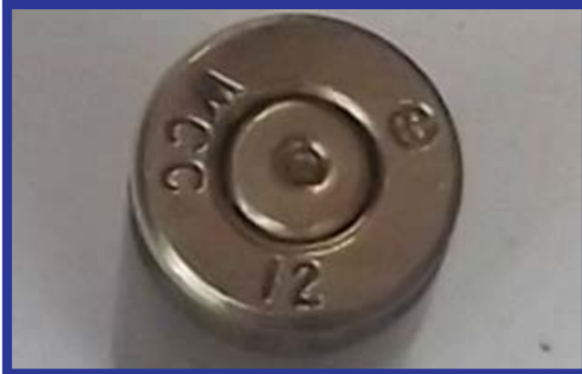
Left: This is 9mm round which has been fired and shows a very good firing pin imprint in the center of the primer. Right: Here is a .22 LR fired case showing the rectangle shape of the firing pin. The thinner shape allows for increased pressure at the point of impact using lighter springs, thus saving production costs. (Photos by Author)
