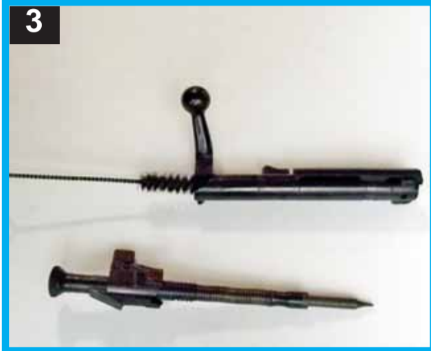
1. When cleaning the bolt or slide of a rifle or pistol use a toothbrush or a brass brush to remove any burnt powder or fouling from the face of the bolt. Also remove any fouling from under the hook of the extractor. The pencil is pointing at the extractor on this bolt. 2. A brass brush works great for removing fouling without removing or damaging the finish. 3. The firing pin should be removed and the firing pin channel cleaned and lightly oiled. 4. The trigger group should not be disassembled except by a gunsmith. However, it needs cleaned also. WD40 and a soft brush works great. (Author Photos)
