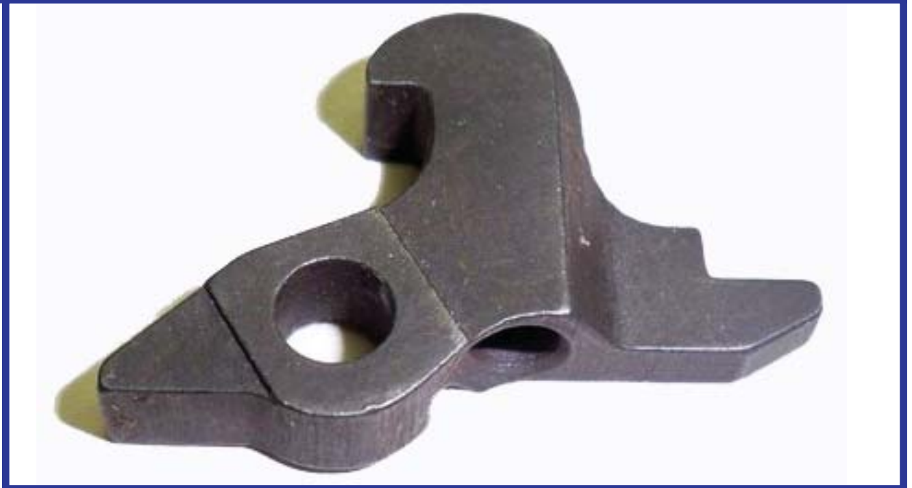
Top Left: The trigger group of the AK-74 in the article. The safety bar has the disconnecter and trigger bar locked in place and safe. Top Right: The safety bar has moved back and is clear of the disconnecter and trigger bar allowing the trigger and disconnect to work. Bottom: This is the disconnecter as used in a AK-74 or AK-47. (Photos by Author)
