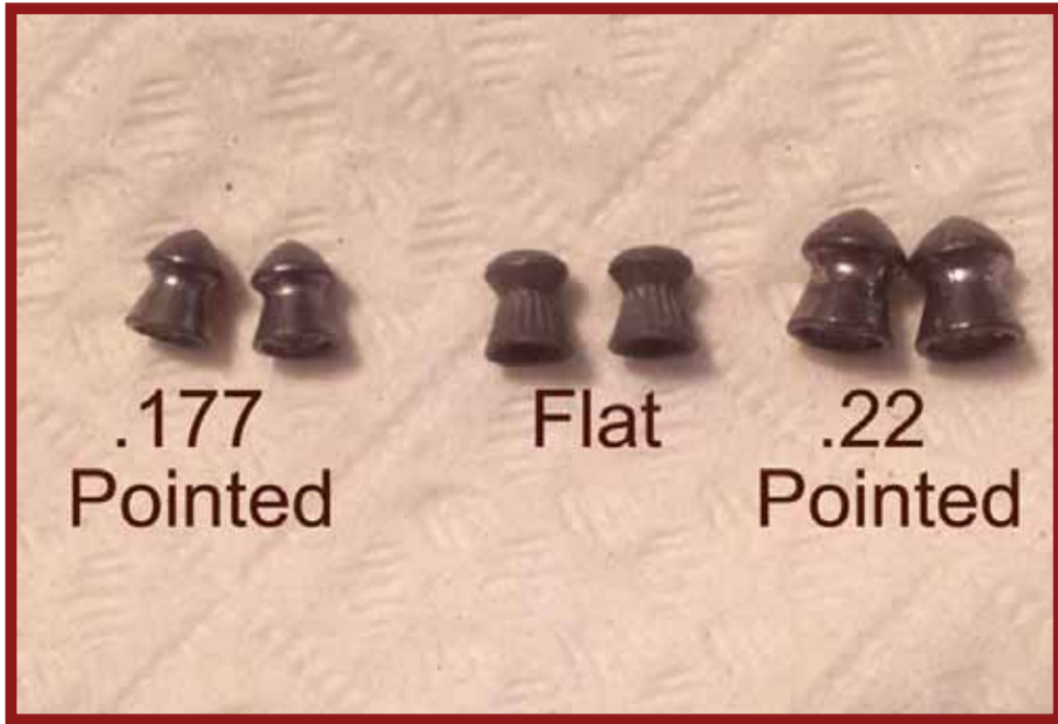
Different sizes of pellets. The pointed .177 lead pellets are 8 grains, the middle flat .177 lead pellet is 6 gr and the right .22 lead pellet is 14 grs. (Author Photo)
