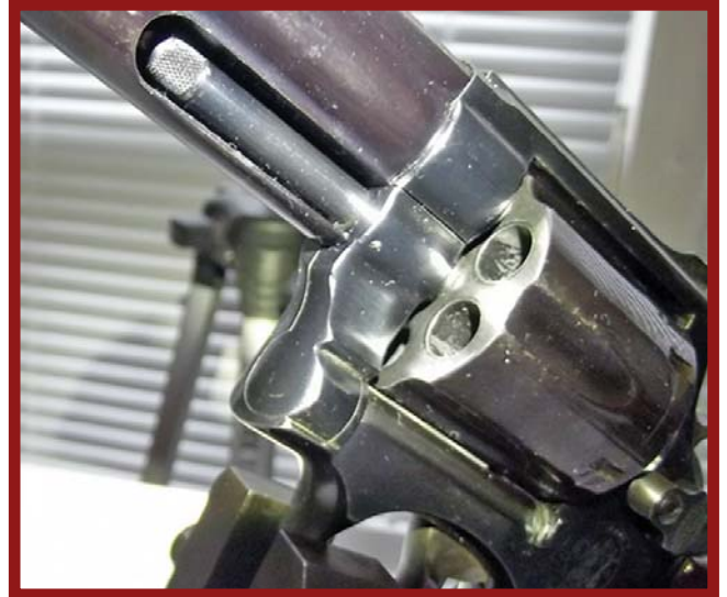
Left Photo: The gun is a S&W Combat Master 586. Notice how the yoke fits to the frame smoothly and evenly. So much so it is hard to define the yoke from the frame. This is how every new and used revolver yoke should fit. Middle Photo: Same gun S&W 586 viewed from the muzzle end. The curvature of the yoke and frame blend smoothly together. This 586 was carried for 14 years on the Police Department. It has had roughly eight or nine thousand rounds fired through it and it still looks and functions like brand new. Well there's a little holster wear on the muzzle and cylinder. Right Photo: The gun shown here is a S&W Model 19-3. It was jammed up and the cylinder wouldn't turn except by hand. Parts, that is the ejector, had apparently been replaced in the the gun and had not been fitted. It also appears the yoke may have been replaced also. The fit of the frame (white line) can be seen standing proud of the yoke and the large gap between the frame and top of the yoke all signs of parts replaced. (Author Photos)
