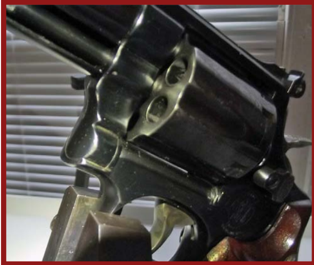
Left Photo: The gun is a S&W Combat Master 586. Notice how the yoke fits to the frame smoothly and evenly. So much so it is hard to define the yoke from the frame. This is how every new and used revolver yoke should fit. Middle Photo: Same gun S&W 586 viewed from the muzzle end. The curvature of the yoke and frame blend smoothly together. This 586 was carried for 14 years on the Police Department. It has had roughly eight or nine thousand rounds fired through it and it still looks and functions like brand new. Well there's a little holster wear on the muzzle and cylinder. Right Photo: The gun shown here is a S&W Model 19-3. It was jammed up and the cylinder wouldn't turn except by hand. Parts, that is the ejector, had apparently been replaced in the the gun and had not been fitted. It also appears the yoke may have been replaced also. The fit of the frame (white line) can be seen standing proud of the yoke and the large gap between the frame and top of the yoke all signs of parts replaced. (Author Photos)
