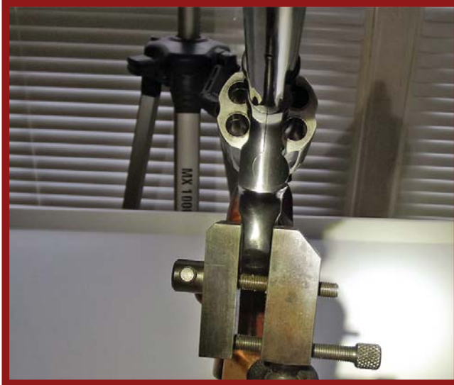
Left Photo: The gun is a S&W Combat Master 586. Notice how the yoke fits to the frame smoothly and evenly. So much so it is hard to define the yoke from the frame. This is how every new and used revolver yoke should fit. Middle Photo: Same gun S&W 586 viewed from the muzzle end. The curvature of the yoke and frame blend smoothly together. This 586 was carried for 14 years on the Police Department. It has had roughly eight or nine thousand rounds fired through it and it still looks and functions like brand new. Well there's a little holster wear on the muzzle and cylinder. Right Photo: The gun shown here is a S&W Model 19-3. It was jammed up and the cylinder wouldn't turn except by hand. Parts, that is the ejector, had apparently been replaced in the the gun and had not been fitted. It also appears the yoke may have been replaced also. The fit of the frame (white line) can be seen standing proud of the yoke and the large gap between the frame and top of the yoke all signs of parts replaced. (Author Photos)
