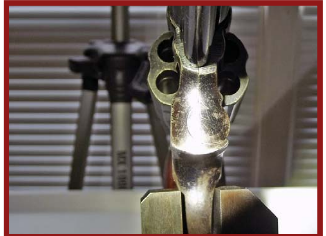
Front view of the 19-3 showing another sign of a replaced yoke. The yoke doesn't blend smoothly into the frame.
