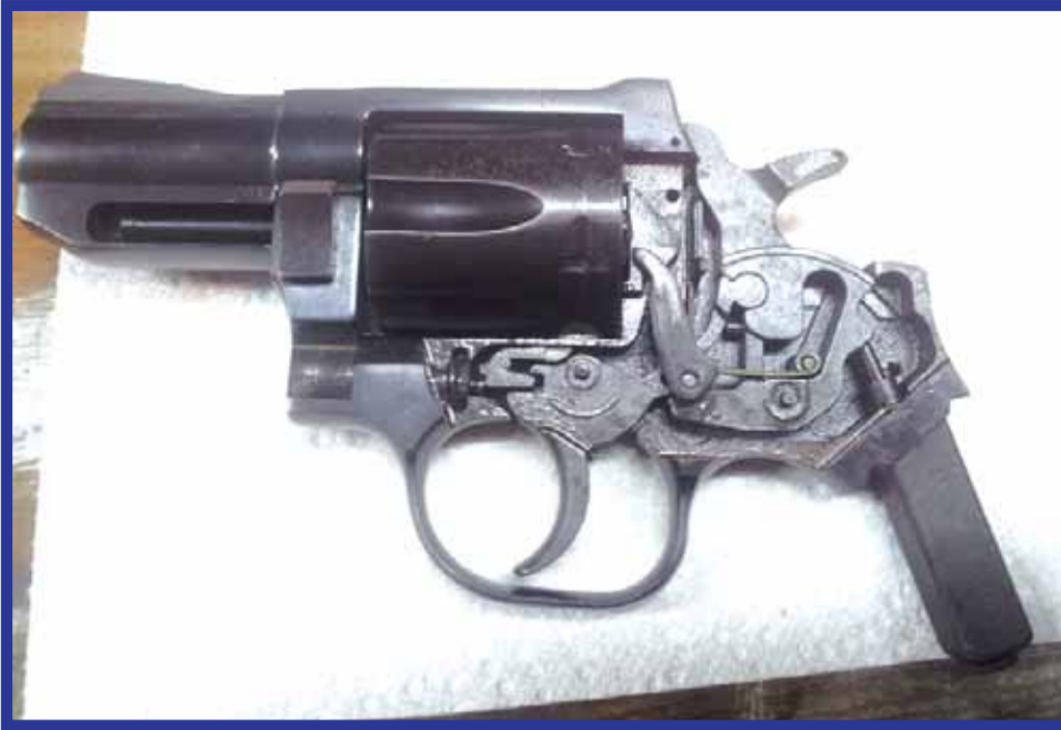
1. This is an example of a revolver with its side plate removed so that the internal working of the parts can be observed. This reduces the time needed to trouble shoot. (Author Photo)
