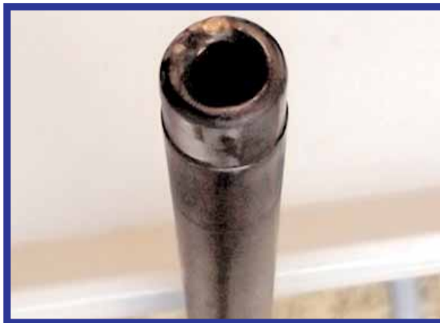
Look closely at the muzzle and you will see a spot on the muzzle crown which has damaged the crown such that a bullet is deflected to the side. This barrel will never shoot accurately until the crown is re-ground. This one was easy to trouble shoot, the damage was obvious. Crowns that have been cut or ground incorrectly may not be easily detected without good and proper information from the gun owner. (Author Photo)
