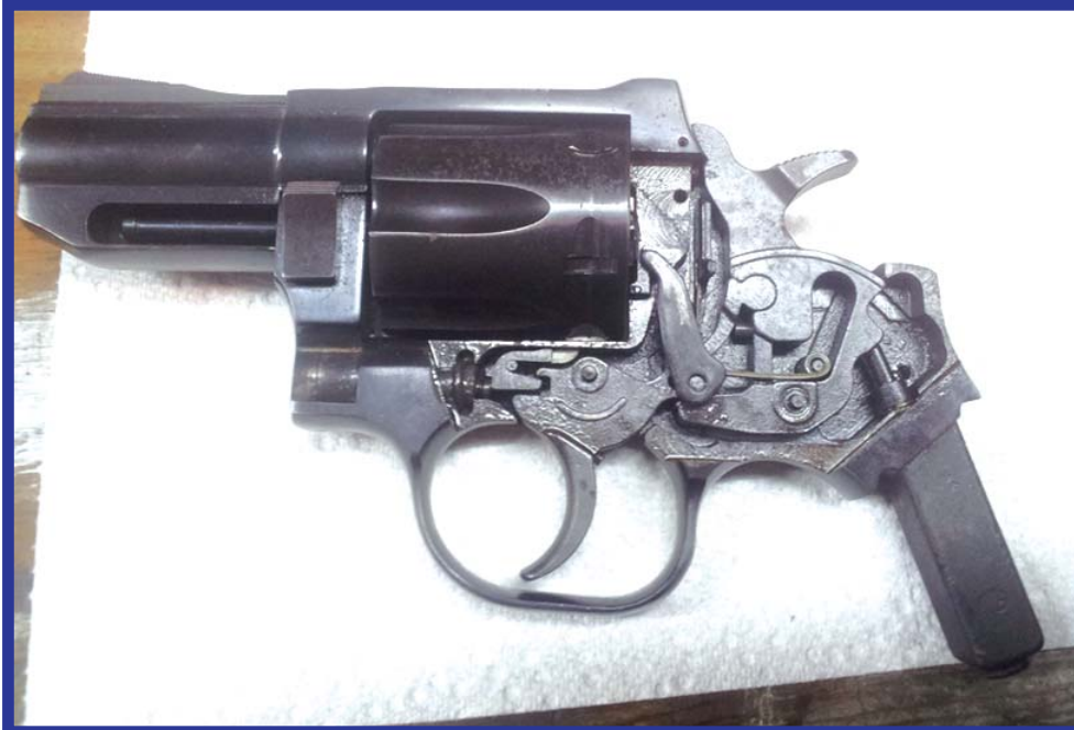
1. This is an example of a revolver with its side plate removed so that the internal working of the parts can be observed. This reduces the time needed to trouble shoot. (Author Photo)
