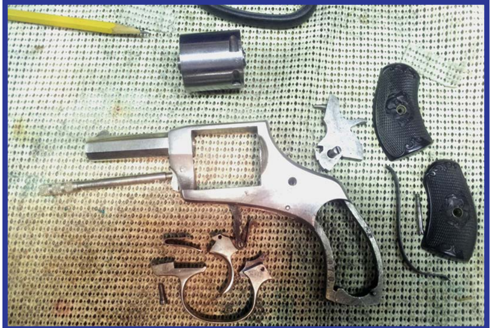
2. An example of the nightmare revolver. All the parts are inside the frame and hidden from view. This type of gun is cheaply made and a nightmare to trouble shoot. (Author Photo)
