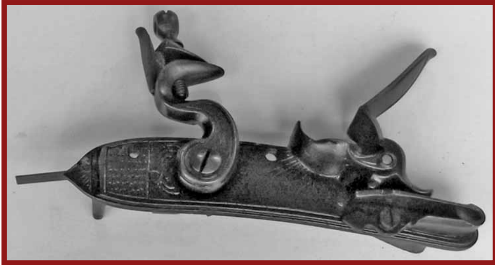
Left Photo: Jukar Black Powder Pistol ready to go home. The frizzen is the leaf like metal plate in front of the hammer and flint. Right Photo: The top is the metal spring material from which the middle piece was made. The middle spring will be heated to red hot and bent in the middle to form the V shape needed for the spring. The bottom is the original spring broken at the bend. (Author Photos)
