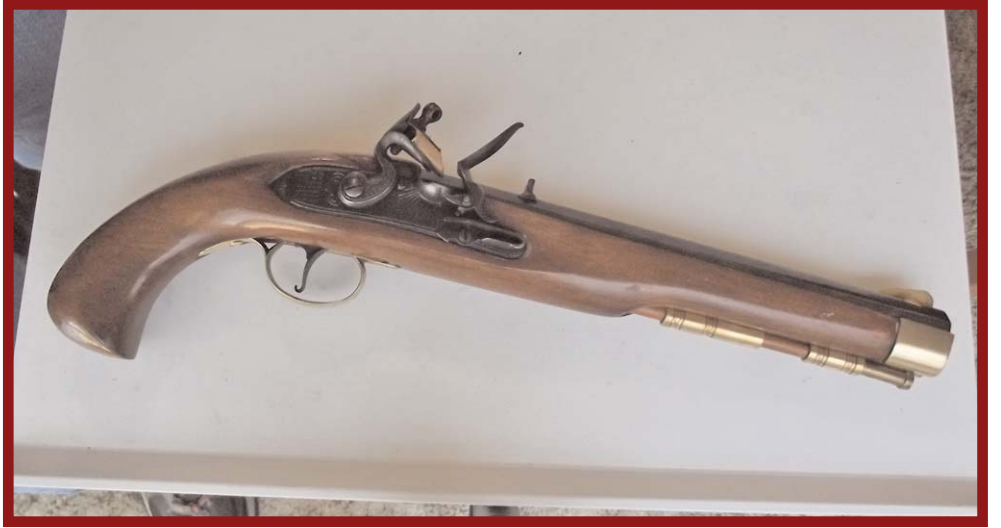
Left Photo: Jukar Black Powder Pistol ready to go home. The frizzen is the leaf like metal plate in front of the hammer and flint. Right Photo: The top is the metal spring material from which the middle piece was made. The middle spring will be heated to red hot and bent in the middle to form the V shape needed for the spring. The bottom is the original spring broken at the bend. (Author Photos)
