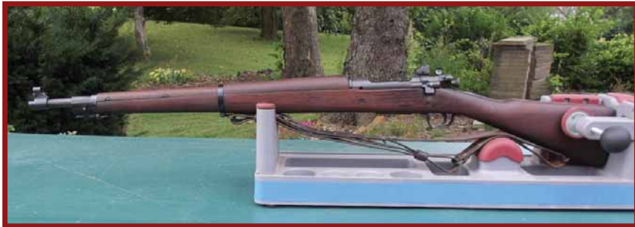
Top Left Photo: This is a Remington 03A3 and the rifle I repaired. It was manufactured by Remington in 1943. The parkerized finish on the barrel was in excellent shape until someone in the past took a torch the muzzle. (Author Photos)
