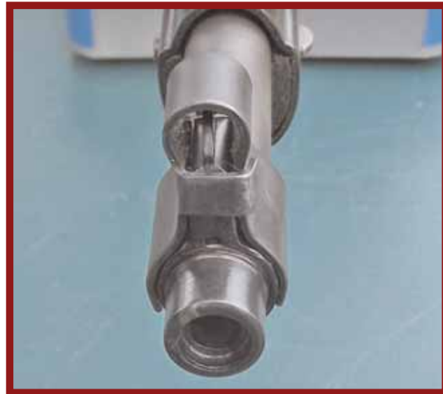
Close up of the muzzle after the sight was removed. The brass material can be seen on the crown and in the bore of the muzzle. Every shot was deflected by the material.
