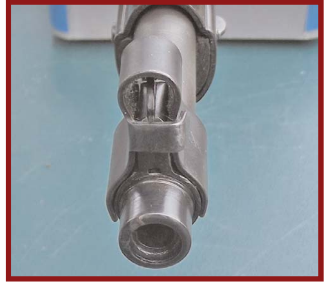
Close up of the muzzle after the sight was removed. The brass material can be seen on the crown and in the bore of the muzzle. Every shot was deflected by the material.
