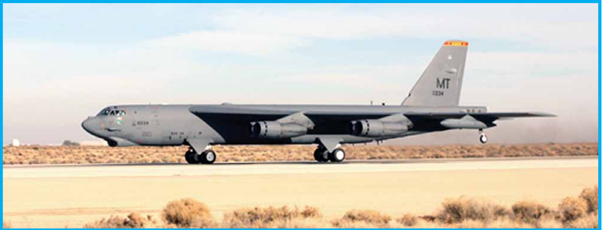
The above photo of this B-52 Stratofortress was the first test flight using a blend of synthetic fuel and JP-8 jet fuel in all eight engines at Edwards Air Force Base on December 15, 2006. The fuel used in all these tests with the B-52 was produced in Tulsa, Oklahoma through the Fischer-Tropsch process that was developed in the 1920s. This flight test was part of the DODs effort to secure domestic sources for our military's energy needs. Further cold weather testing was scheduled for the new alternative fuel source. (USAF Photo)
