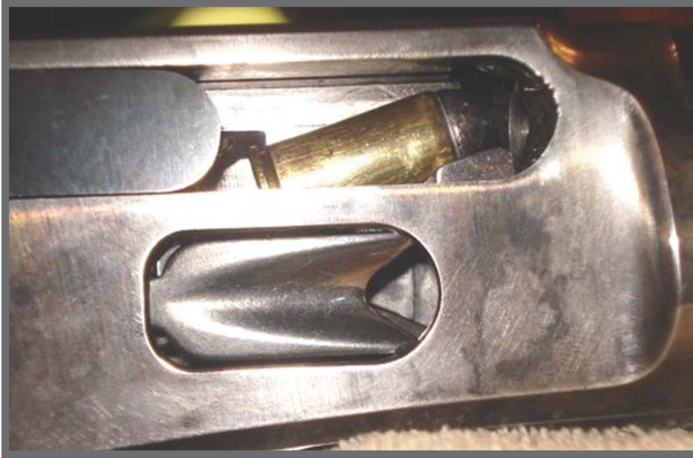
This is a view of how the cartridge is lifted and slid under the extractor in a lever action gun. If the point of the extractor is not cut at an angle it can gouge into the brass as it appears to be doing and cause a failure to feed. (This picture is from the internet at http://marauder.homestead.com/files/Widdermajic_Marlin.htm )
