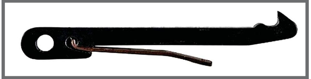
Here the bottom side of the Marlin 93 extractor is shown and the lighter area under the tip of the extractor is where it is chamfered. However, I had to round the edge of the shaft on a Marlin 93 extractor as it was cutting into brass rim of a .44 Mag as it was sliding into the chamber causing a failure to feed. (Picture is from Midway USA online catalog)
