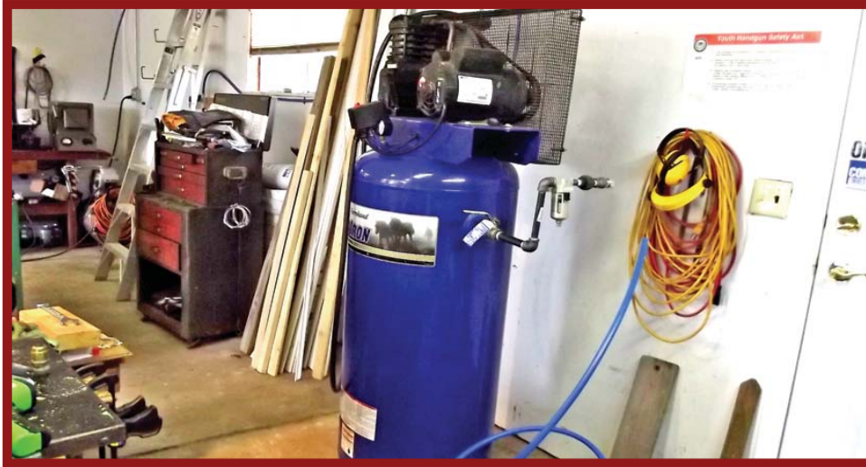
Left Photo: My new to me air compressor. I installed the ball valve and Water/oil trap. The blue tubing on the floor is a pex-al 1/2 inch tubing which should carry all the air I'll need. It is easy to install and bends holding its shape without a tube bender. Just don't make a bend with less than an 8" radius. Right Photo: "I've installed some of the tubing and am locating the stations. There will be 3 regulated stations and one unregulated." (Author Photos)
