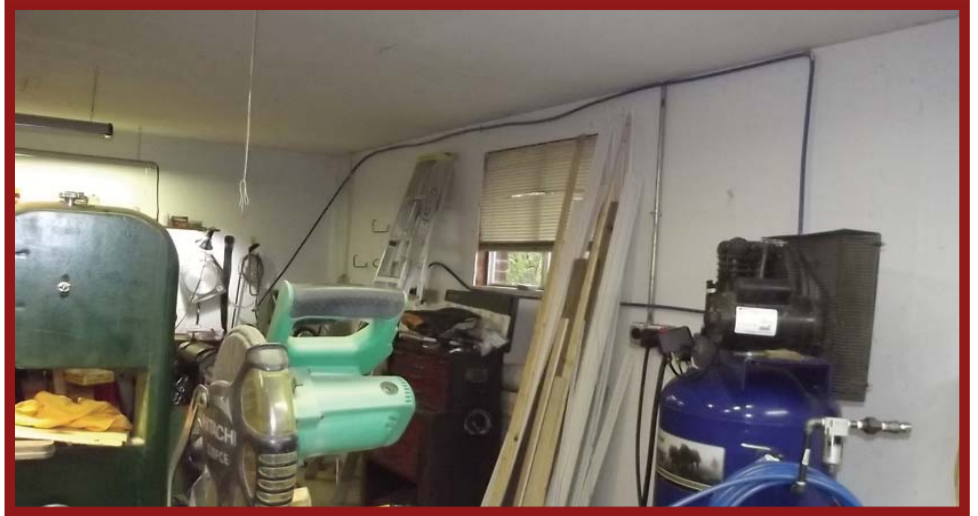
Left Photo: My new to me air compressor. I installed the ball valve and Water/oil trap. The blue tubing on the floor is a pex-al 1/2 inch tubing which should carry all the air I'll need. It is easy to install and bends holding its shape without a tube bender. Just don't make a bend with less than an 8" radius. Right Photo: "I've installed some of the tubing and am locating the stations. There will be 3 regulated stations and one unregulated." (Author Photos)
