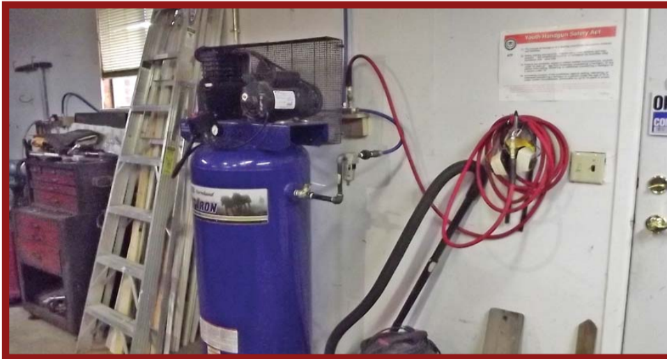
Left Photo: Finally installed and running. It took a couple of more days to chase down leaks and tighten all the leaky fittings. Right Photo: After 24 years of service I hate to get rid of the old compressor. I'm going to have to think of how I can re-purpose the good parts. The motor seems good, the pressure switch and regulator seems okay, and the tank appears solid. I'll be thinking about that. (Author Photos)
