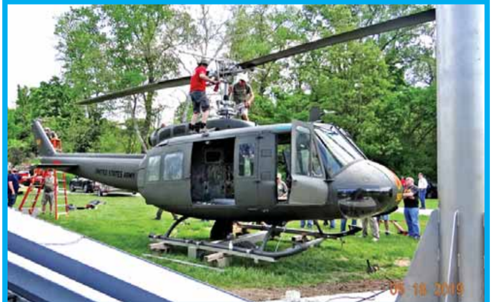
Left Photo: Charley Walker keeps an eye on the progress of installing rotor assembly in top of Huey. The Crane operator assists in this very important assembly process. Right Photo: Charley Walker and Vietnam Veteran working on main rotor as other Veterans work on tail rotor. These are the final stages and last before placing the Huey on tower.
