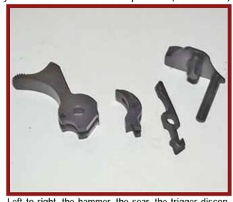
Left to right, the hammer, the sear, the trigger disconnect, and the manual external safety. All of these parts will need to be replaced to make the gun safe and avoid the safety issues of the untempered hammer and sear. The trigger disconnect and manual safety will have to be replaced and tuned to the hammer and sear. (Author
