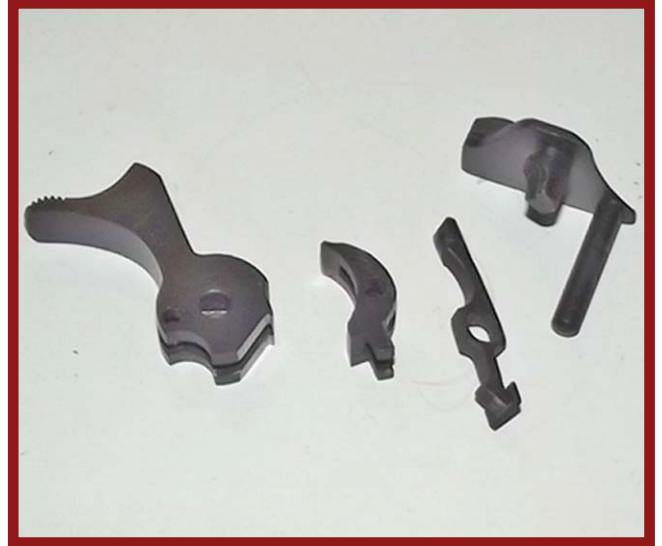
Left to right, the hammer, the sear, the trigger disconnect, and the manual external safety. All of these parts will need to be replaced to make the gun safe and avoid the safety issues of the untempered hammer and sear. The trigger disconnect and manual safety will have to be replaced and tuned to the hammer and sear. (Author Photo)
