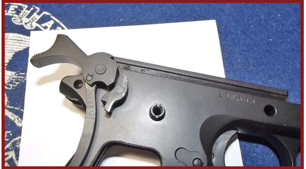
The hammer and sear as they should connect in the cocked position. (Author Photo)
