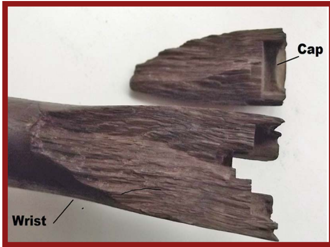
Left Photo: Here the rotational action of the recoil on an oil soaked and weakened pistol grip stock has cracked and then broken the cap of the wrist off the pistol grip stock. This is from a 12 ga. Pump shotgun. Center Photo: This is a closeup view of the cap and stock break. The picture doesn't give a very good view of the oil soaked end of the stock. It does show the grain of the stock which is in line with the recoil direction and not giving a stronger stock in that area. If the grain of the stock were more diagonal to the direction of the recoil there would be less chance of the wrist cracking even when weakened by the oil from the gun. Right Photo: This old double barrel external hammer shotgun stock has extensive cracking in the straight grip receiver cutout. Mostly due to the years of oil soaking the wood and continued pounding from the recoil. The white is the expanding glue used to reinforce the grip and hold the piece together. The gun is a wall hanger and won't be shot. If the intention was to put the gun back in the field then a new stock would be required. Bottom Right Photo: This is an antique external hammer L.C. Smith double coach gun with Damascus Steel Barrels. The wood has split at both the top and bottom of the wrist where the action came loose and the recoil movement cracked the stock's "ears". The cracks will be glued back in place and the finish redone to match the original. This will make a beautiful presentation (aka: Wall Hanger) gun when done. (Author Photos)
