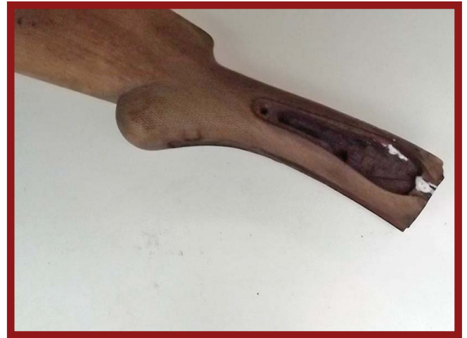
Left Photo: Here the rotational action of the recoil on an oil soaked and weakened pistol grip stock has cracked and then broken the cap of the wrist off the pistol grip stock. This is from a 12 ga. Pump shotgun. Center Photo: This is a closeup view of the cap and stock break. The picture doesn't give a very good view of the oil soaked end of the stock. It does show the grain of the stock which is in line with the recoil direction and not giving a stronger stock in that area. If the grain of the stock were more diagonal to the direction of the recoil there would be less chance of the wrist cracking even when weakened by the oil from the gun. Right Photo: This old double barrel external hammer shotgun stock has extensive cracking in the straight grip receiver cutout. Mostly due to the years of oil soaking the wood and continued pounding from the recoil. The white is the expanding glue used to reinforce the grip and hold the piece together. The gun is a wall hanger and won't be shot. If the intention was to put the gun back in the field then a new stock would be required. Bottom Right Photo: This is an antique external hammer L.C. Smith double coach gun with Damascus Steel Barrels. The wood has split at both the top and bottom of the wrist where the action came loose and the recoil movement cracked the stock's "ears". The cracks will be glued back in place and the finish redone to match the original. This will make a beautiful presentation (aka: Wall Hanger) gun when done. (Author Photos)
