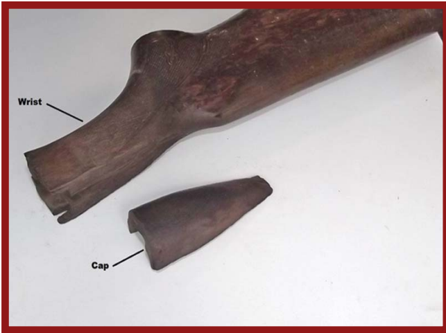
Left Photo: Here the rotational action of the recoil on an oil soaked and weakened pistol grip stock has cracked and then broken the cap of the wrist off the pistol grip stock. This is from a 12 ga. Pump shotgun. Center Photo: This is a closeup view of the cap and stock break. The picture doesn't give a very good view of the oil soaked end of the stock. It does show the grain of the stock which is in line with the recoil direction and not giving a stronger stock in that area. If the grain of the stock were more diagonal to the direction of the recoil there would be less chance of the wrist cracking even when weakened by the oil from the gun. Right Photo: This old double barrel external hammer shotgun stock has extensive cracking in the straight grip receiver cutout. Mostly due to the years of oil soaking the wood and continued pounding from the recoil. The white is the expanding glue used to reinforce the grip and hold the piece together. The gun is a wall hanger and won't be shot. If the intention was to put the gun back in the field then a new stock would be required. Bottom Right Photo: This is an antique external hammer L.C. Smith double coach gun with Damascus Steel Barrels. The wood has split at both the top and bottom of the wrist where the action came loose and the recoil movement cracked the stock's "ears". The cracks will be glued back in place and the finish redone to match the original. This will make a beautiful presentation (aka: Wall Hanger) gun when done. (Author Photos)
