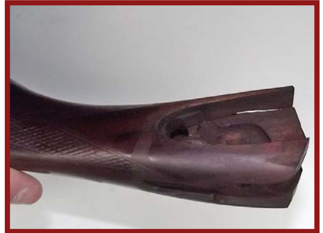
Left Photo: Here the rotational action of the recoil on an oil soaked and weakened pistol grip stock has cracked and then broken the cap of the wrist off the pistol grip stock. This is from a 12 ga. Pump shotgun. Center Photo: This is a closeup view of the cap and stock break. The picture doesn't give a very good view of the oil soaked end of the stock. It does show the grain of the stock which is in line with the recoil direction and not giving a stronger stock in that area. If the grain of the stock were more diagonal to the direction of the recoil there would be less chance of the wrist cracking even when weakened by the oil from the gun. Right Photo: This old double barrel external hammer shotgun stock has extensive cracking in the straight grip receiver cutout. Mostly due to the years of oil soaking the wood and continued pounding from the recoil. The white is the expanding glue used to reinforce the grip and hold the piece together. The gun is a wall hanger and won't be shot. If the intention was to put the gun back in the field then a new stock would be required. Bottom Right Photo: This is an antique external hammer L.C. Smith double coach gun with Damascus Steel Barrels. The wood has split at both the top and bottom of the wrist where the action came loose and the recoil movement cracked the stock's "ears". The cracks will be glued back in place and the finish redone to match the original. This will make a beautiful presentation (aka: Wall Hanger) gun when done. (Author Photos)
