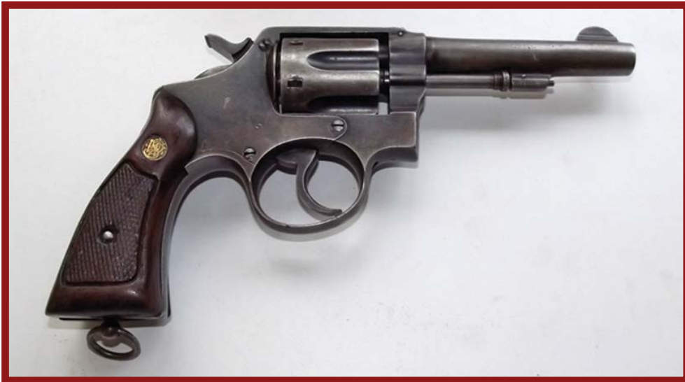
Trocaola Aranzabal Y Cia Eibar, made in Spain also called the French Model 1892 or just 92. Note the lanyard ring on the grip frame. That's a good indication of military use. Author's Photo
