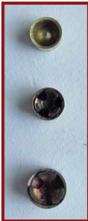
Left Photo: The firing pin was striking the round with just enough force to lightly dent the primer but not detonate. Center Photo: Top empty primer cup—When I looked into the now empty case I could see that the primer cup was well dented but was missing the primer charge and the anvil. Just an empty primer cup. Middle—Fired primer with anvil, Bottom—Unfired Primer with anvil. Right Photo: The print on the barrel was so small I mistook it for 9mm Luger. Only a magnifying glass showed it to be Largo. (Author Photos)
