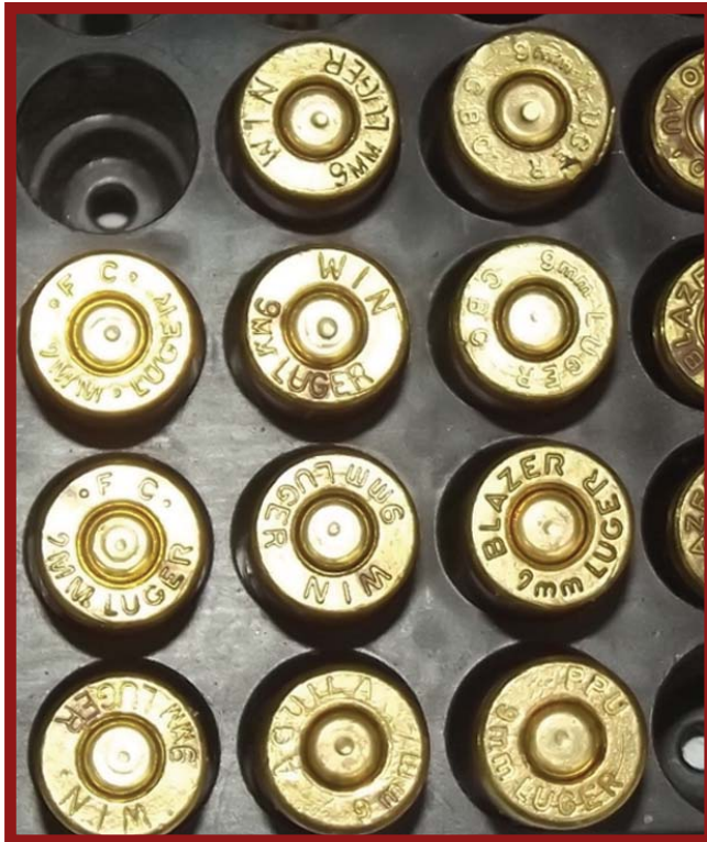
Left Photo: The firing pin was striking the round with just enough force to lightly dent the primer but not detonate. Center Photo: Top empty primer cup—When I looked into the now empty case I could see that the primer cup was well dented but was missing the primer charge and the anvil. Just an empty primer cup. Middle—Fired primer with anvil, Bottom—Unfired Primer with anvil. Right Photo: The print on the barrel was so small I mistook it for 9mm Luger. Only a magnifying glass showed it to be Largo. (Author Photos)
