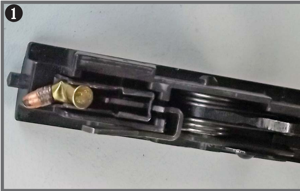
How the bullet got bent in a 90 degree angle and lodged in the trigger housing is a real head scratcher. (Author Photo).
