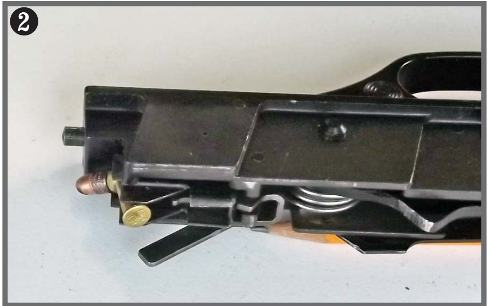
Had the base of the bullet been a few thousandths higher the bolt would have struck the primer set the round off most likely injuring someone severely. (Author Photo).
