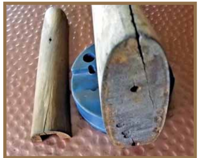
The crack in the toe of the stock extends for about 3 inches up through the butt towards the heel of the stock. (Author Photo)
