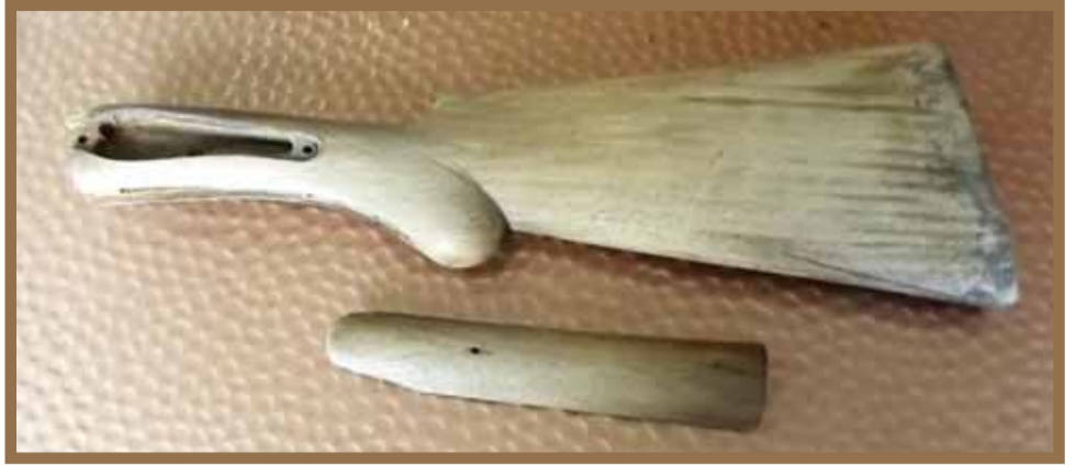
I've had to soak the stock in lacquer thinner for several months to get as much oil out as possible and then let it dry for a few more months to get the cracks to settle down. After having been soaked the cracks had opened up like the Grand Canyon. It's now been 9 months and the stock appears that it may be ready to work. (Author Photo)
