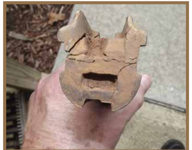
The crack in the top of the grip just behind the receiver tang will also be epoxied to close it up. (Author Photo)
