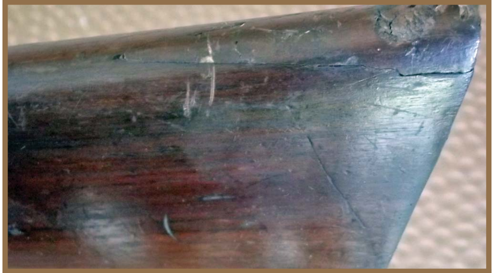
Top Left Photo: The only problems with disassembly was the rusted and frozen barrel band screws. I don't think the picture shows the extent of the exterior rust very well. The color of the table blends into the color of the rust. Top Right Photo: My experience has been that when the toe of the stock cracks and comes apart from the rest of the stock it's due to someone tightening the butt plate screw that is too large for the hole and expanding the wood causing it to crack along the grain of the wood. Bottom Right Photo: The bore had a fine layer of rust but cleaned up nicely. There was a layer of leading which indicated to me that the gun had a lot of use over the years. (Author Photo)
