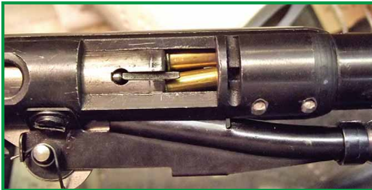
"Shown is a Springfield Model 187. It is jammed with what looks like a double feed problem but it was a broken ejector. The extractor is just above the bottom cartridge which is sliding up to engage the extractor and enter the rifle chamber. The upper cartridge is the spent round which the ejector pulled free from the chamber but did not get bumped out of the receiver by the ejector which had broken. Once jammed like this it may take a complete disassembly to remove the two rounds." (Author Photo)
