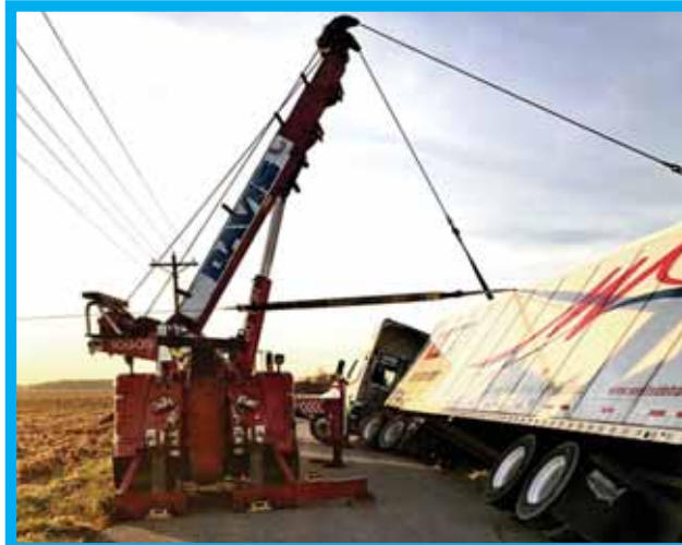
Davis Recovery crew righting an overturned semi-trailer. (Davis Towing & Recovery Photo)
