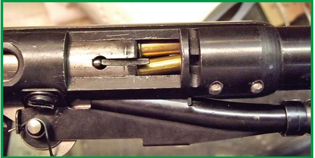
"Shown is a Springfield Model 187. It is jammed with what looks like a double feed problem but it was a broken ejector. The extractor is just above the bottom cartridge which is sliding up to engage the extractor and enter the rifle chamber. The upper cartridge is the spent round which the ejector pulled free from the chamber but did not get bumped out of the receiver by the ejector which had broken. Once jammed like this it may take a complete disassembly to remove the two rounds." (Author Photo)
