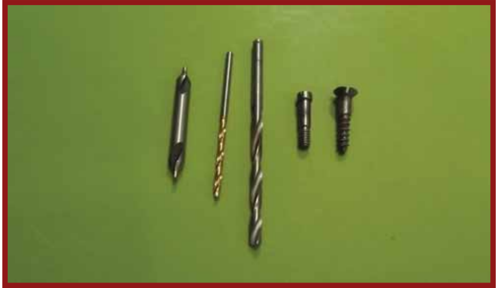
Left: In this picture I have drilled out the damaged plugs on both firing pins and re-tapped them to accept a 6-48 plug. The plug needs to be about 7/16" long and looks like I'll have to make them as that thread in a #6 plug with a slotted plug. I'll make it from 6-48x1/2" slotted scope mount screws. I will cut the screw heads down to size to fit like the originals. I haven't done that at the time of this article. Right: From left to right is a center drill, a #30 drill bit, a 7/64" drill bit to remove the head of the screw, a shoulder screw, and on the right a butt plate wood screw. This particular butt plate screw was so rusted into the stock that the stock split when the screw was forced out. (Author Photos)
