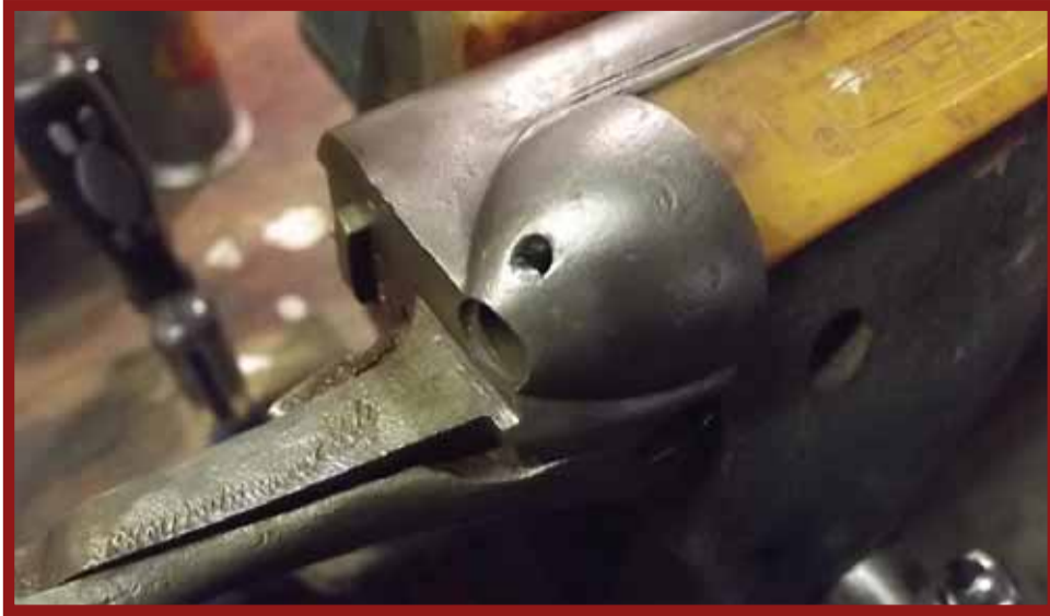
Left: In this picture I have drilled out the damaged plugs on both firing pins and re-tapped them to accept a 6-48 plug. The plug needs to be about 7/16" long and looks like I'll have to make them as that thread in a #6 plug with a slotted plug. I'll make it from 6-48x1/2" slotted scope mount screws. I will cut the screw heads down to size to fit like the originals. I haven't done that at the time of this article. Right: From left to right is a center drill, a #30 drill bit, a 7/64" drill bit to remove the head of the screw, a shoulder screw, and on the right a butt plate wood screw. This particular butt plate screw was so rusted into the stock that the stock split when the screw was forced out. (Author Photos)
