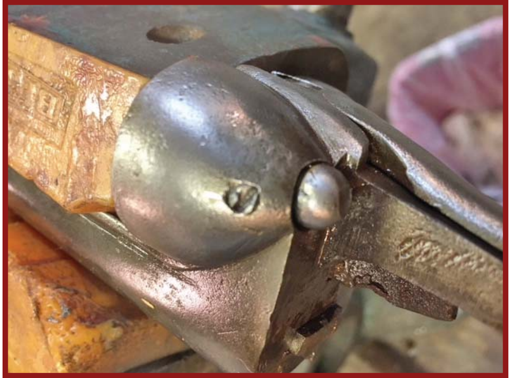
Left: This screw holds the right firing pin (missing) and is of soft iron, and, rusted into place, the screwdriver forced edges of the screw out and over the edges of the screw hole. After a lot of soaking in penetrating oil, and peening with a hammer it still refused to budge and had to be drilled out. I'll have more on that next month. Right: This screw holds the right firing pin (missing) and is of soft iron, and, rusted into place, the screwdriver forced edges of the screw out and over the edges of the screw hole. After a lot of soaking in penetrating oil, and peening with a hammer it still refused to budge and had to be drilled out. I'll have more on that next month. (Author Photos)
