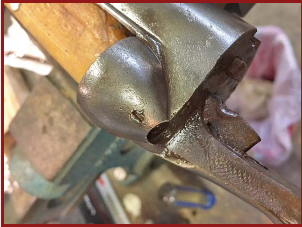
Left: This screw holds the right firing pin (missing) and is of soft iron, and, rusted into place, the screwdriver forced edges of the screw out and over the edges of the screw hole. After a lot of soaking in penetrating oil, and peening with a hammer it still refused to budge and had to be drilled out. I'll have more on that next month. Right: This screw holds the right firing pin (missing) and is of soft iron, and, rusted into place, the screwdriver forced edges of the screw out and over the edges of the screw hole. After a lot of soaking in penetrating oil, and peening with a hammer it still refused to budge and had to be drilled out. I'll have more on that next month. (Author Photos)
