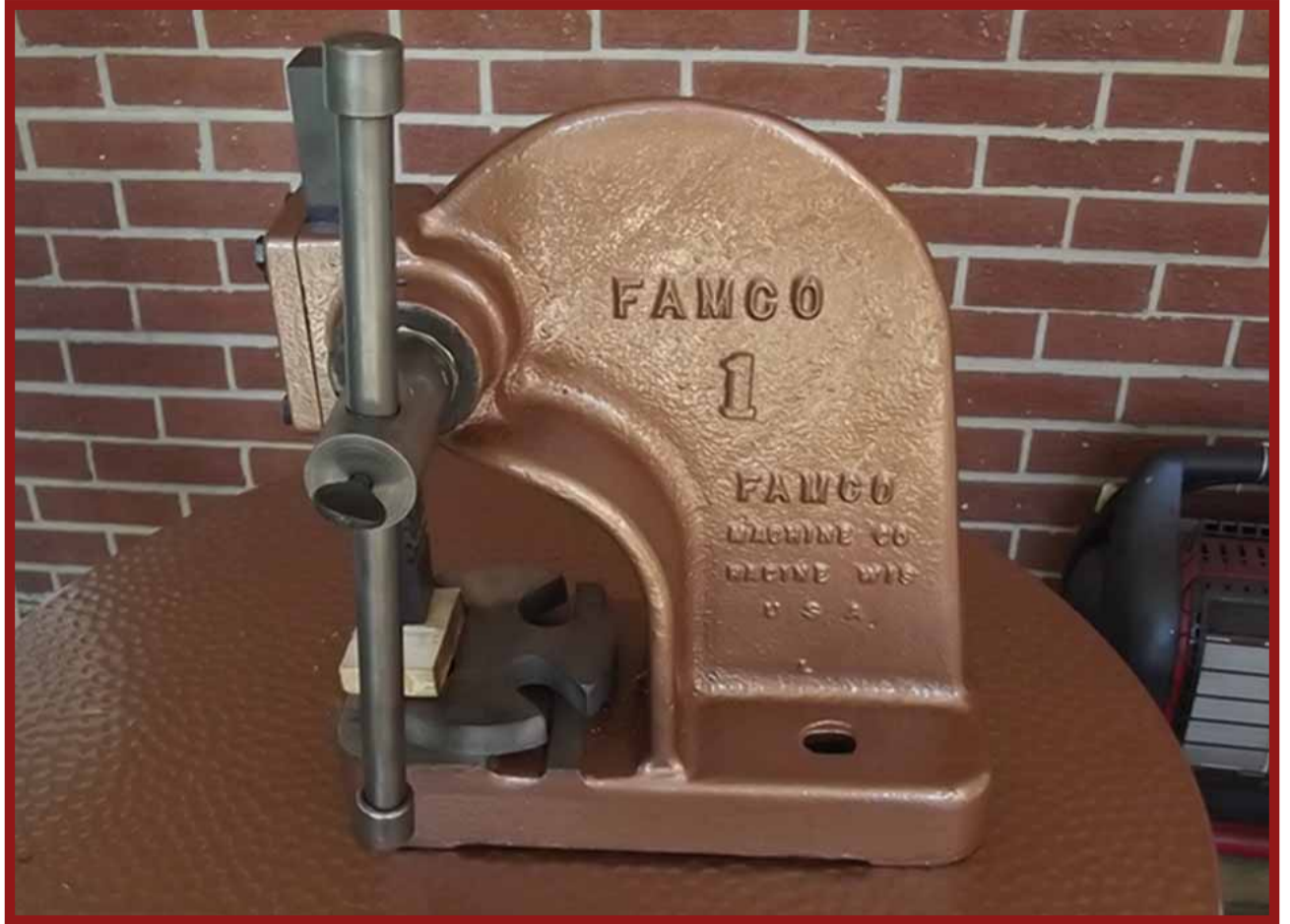
Left Photo: FAMCO Arbor Press before cleaning and painting. Right Photo: FAMCO Machine Co. of Racine, Wisconsin 1 ton Arbor Press. I have used the press about a dozen times in the past month to press out stubborn pins in guns and to remove the small gear on the threading dial on my small Craftsman 6" lathe. (Author Photos)
