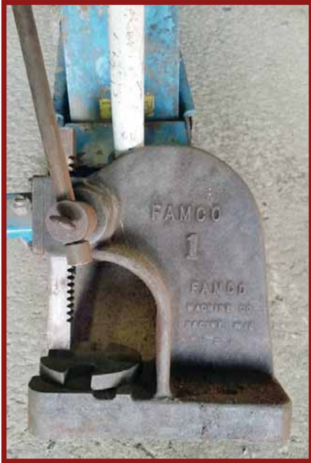
Left Photo: FAMCO Arbor Press before cleaning and painting. Right Photo: FAMCO Machine Co. of Racine, Wisconsin 1 ton Arbor Press. I have used the press about a dozen times in the past month to press out stubborn pins in guns and to remove the small gear on the threading dial on my small Craftsman 6" lathe. (Author Photos)
