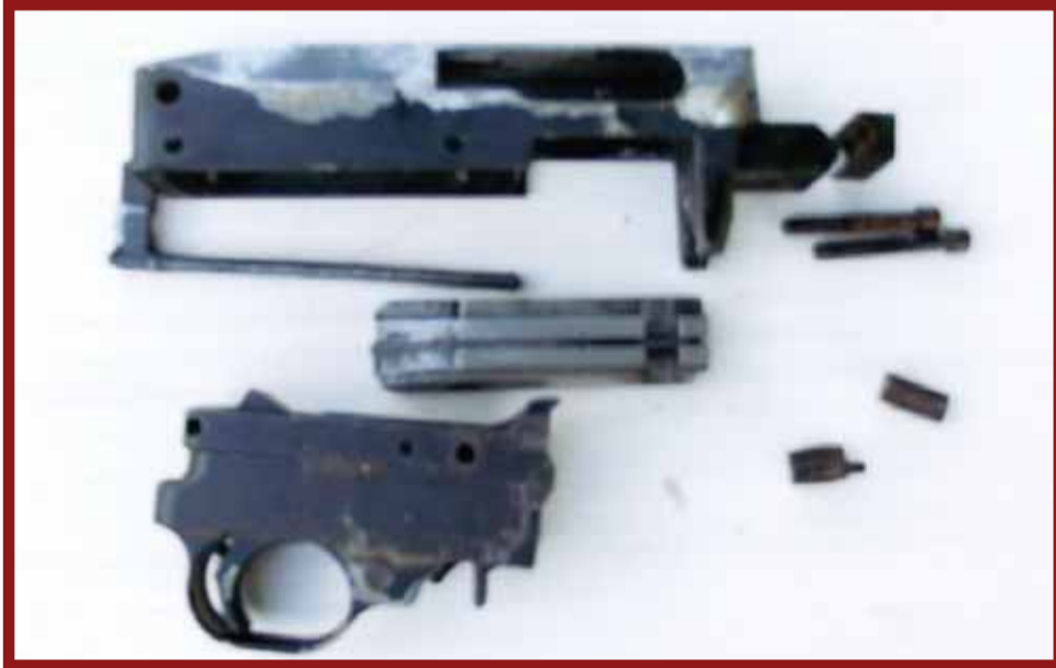
Left Photo: A disassembled view of the internals of the 10-22. Some will get blued, others I'll leave in the white. Right Photo: A look down the barrel of the 10-22. It looks to be in good shape. No rust or pits. Hopefully, it will be a fine shooter. (Author Photos)
