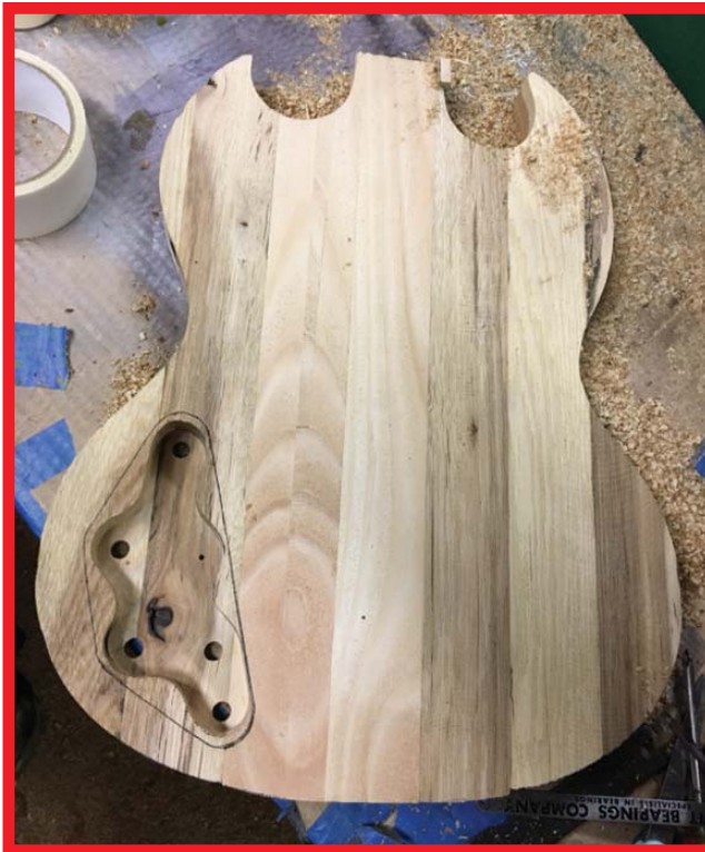
Left Photo: The raw guitar body from a back view with routed insets for volume controls. Right Photo: The guitar body glued together ready for assembly. (Author Photos)
