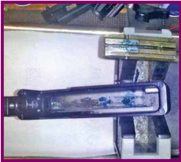
Left Photo: Here is a picture of the blue Loctite® inside the receiver and on the bolt. Center Photo: This is the bolt and firing pin. The pin was cemented inside the bolt and wouldn't budge. Heat was needed to loosen the firing pin for removal. Right Photo: This picture is looking down into the trigger group. The blue loctite has migrated onto the top of the hammer. Luckily it had not gotten further into the trigger group. (Author Photos)
