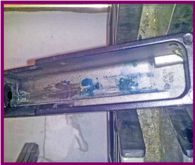
This is looking into the receiver with the bolt and trigger group removed. It's easy to see the 4 screws and where the blue Loctite® has hardened wedging the bolt and receiver together. (Author Photo)
