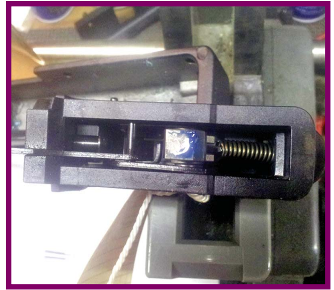
Left Photo: Here is a picture of the blue Loctite® inside the receiver and on the bolt. Center Photo: This is the bolt and firing pin. The pin was cemented inside the bolt and wouldn't budge. Heat was needed to loosen the firing pin for removal. Right Photo: This picture is looking down into the trigger group. The blue loctite has migrated onto the top of the hammer. Luckily it had not gotten further into the trigger group. (Author Photos)
