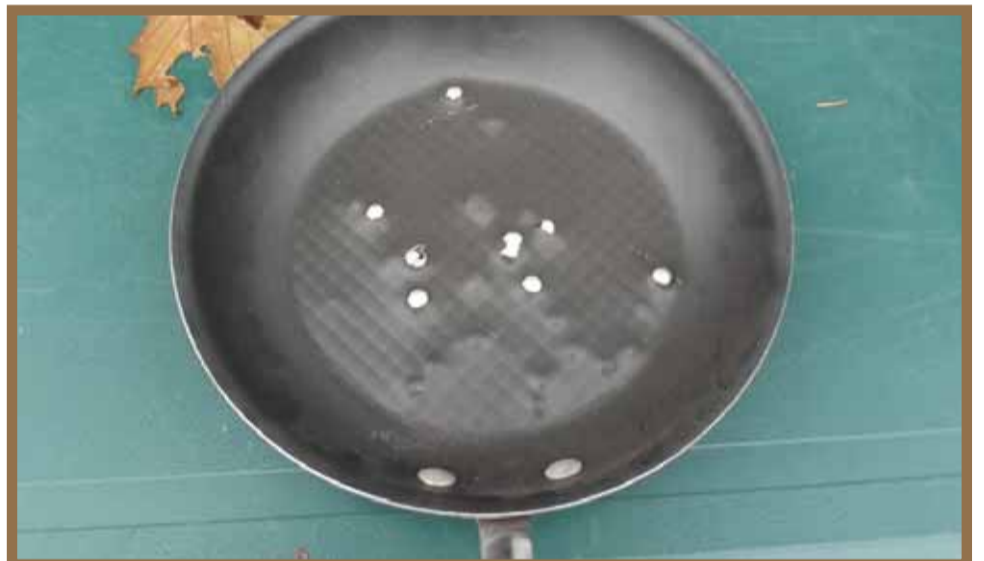
Left Photo: The dents in the bottom of this aluminum fry pan tell the story. Those bright spots are where the oil treated pellets struck and embedded themselves into the bottom of the pan. Looking closely one can even see the ring of the inside of the pellet that has flattened out. Right Photo: After testing was completed I found that one pellet struck with such force that it penetrated and passed through the aluminum bottom of the pan. It's at the 9 o'clock position where the aluminum is standing proud of the pan. (Author Photos)
