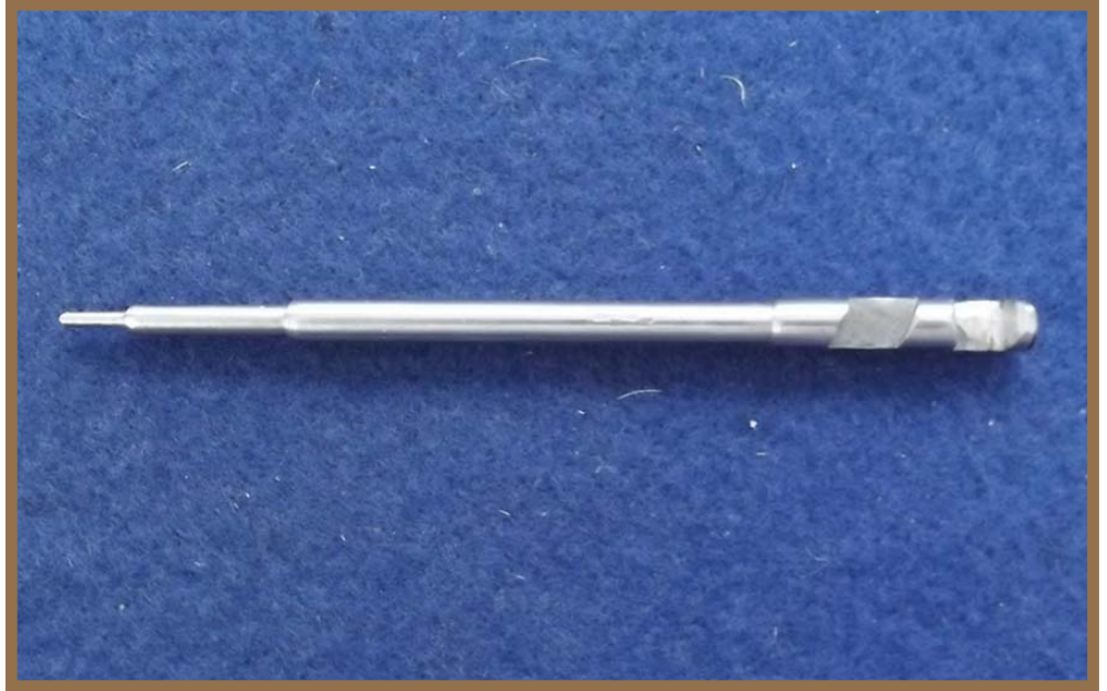
Ah, the final product. I decided not to harden the firing pin. The drill rod used is already hard enough and heat treating it would make it too brittle. Anyway, I like it shiny. (Author Photo)
