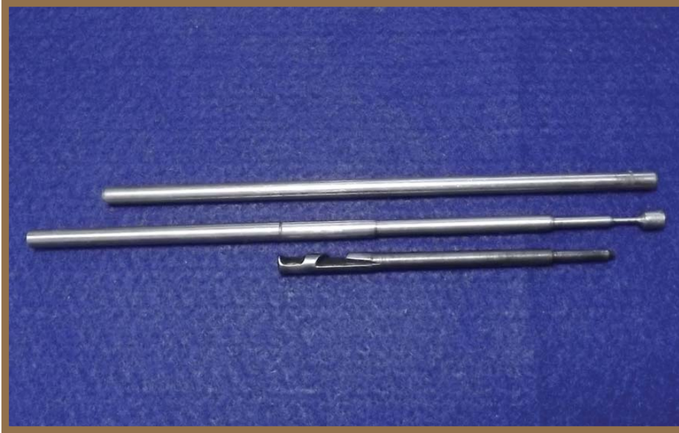
The top is the blank drill rod I chose to make the firing pin with. The Middle pin is the initial turning of the pin. Note the large portion on the right end of the pin, it is left on to support the smaller diameter of the pin to avoid breaking the work piece. The bottom is the original firing pin less its tip. This is what I am copying. (Author Photo)
