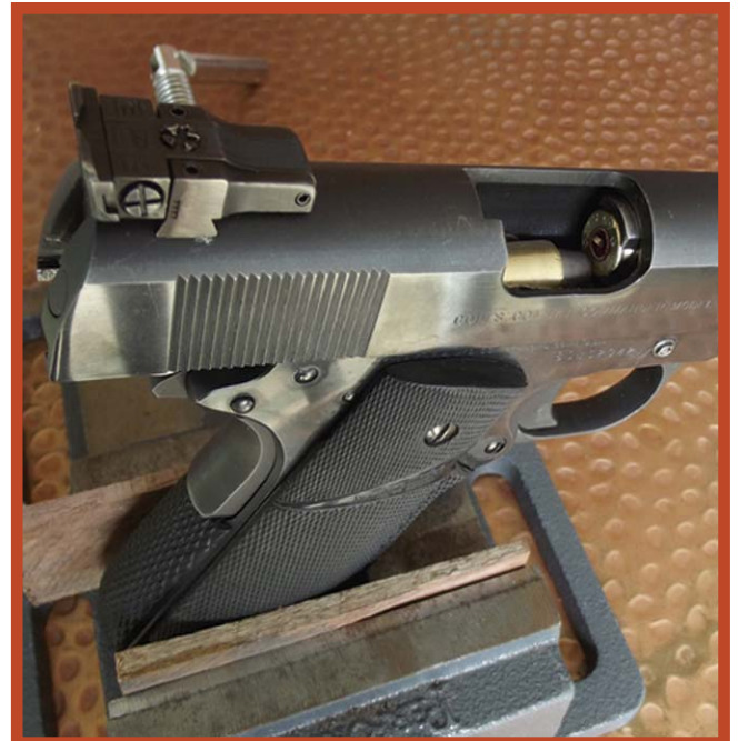
Left Photo: Failure to feed (FTF), this is symptomatic of short stroking. The round in the chamber has been ejected but the round in the magazine hasn't been picked up and the slide is trying to go into battery but didn't pick up the round in the magazine at the head of the bullet and is now caught half way up the cartridge. Middle Photo: Failure to eject (FTE), this stove pipe jam is another indicator of short stroking. There wasn't enough recoil power to eject the spent case or to pick up the next round. Right Photo: Failure to extract (FTX), this is called a double feed and it is a failure to extract. The gun's extractor wasn't able to grab or hold the cartridge's rim. If not broken, the extractor may be dirty and standing away from the cartridge rim or stuck in its channel. Clearing this malfunction may be hard. The magazine may not release and the jammed bullet will have to be removed or pushed back into the magazine before you can clear the gun. A good cleaning will usually cure this problem. (Author Photos)
