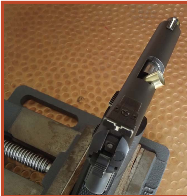
Left Photo: Failure to feed (FTF), this is symptomatic of short stroking. The round in the chamber has been ejected but the round in the magazine hasn't been picked up and the slide is trying to go into battery but didn't pick up the round in the magazine at the head of the bullet and is now caught half way up the cartridge. Middle Photo: Failure to eject (FTE), this stove pipe jam is another indicator of short stroking. There wasn't enough recoil power to eject the spent case or to pick up the next round. Right Photo: Failure to extract (FTX), this is called a double feed and it is a failure to extract. The gun's extractor wasn't able to grab or hold the cartridge's rim. If not broken, the extractor may be dirty and standing away from the cartridge rim or stuck in its channel. Clearing this malfunction may be hard. The magazine may not release and the jammed bullet will have to be removed or pushed back into the magazine before you can clear the gun. A good cleaning will usually cure this problem. (Author Photos)
