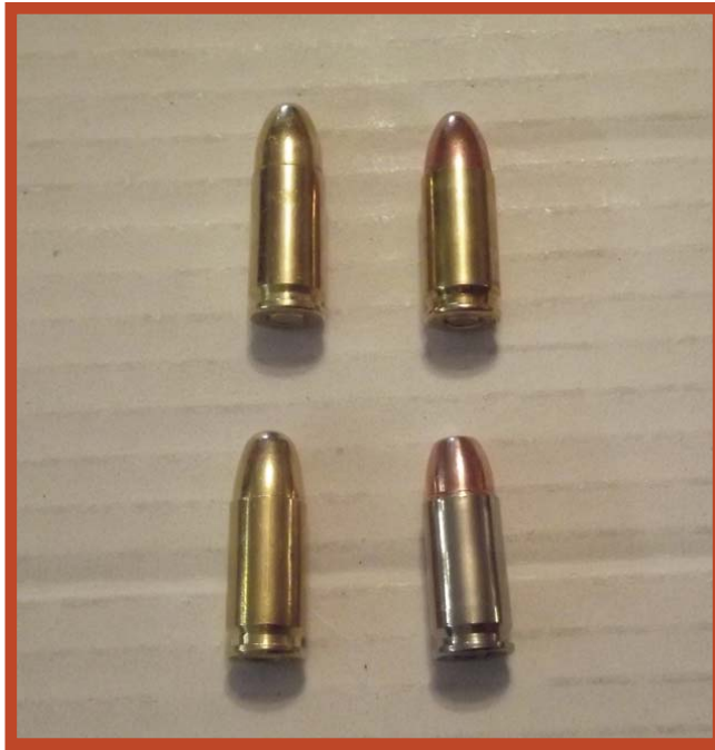
Left picture has 4 cartridges base up. Right picture is the same bullets in side view. Upper left is a S&B 9x19 mm (Sellier & Bellot), Lower Left is a Tulammo 9mm Luger, both weigh 184 grains, OAL is the same and look like the same cartridge. Upper right is a R-P 9mm Luger, it is shorter and weighs less than the S&B or Tulammo. Lower right is a Speer 9mm Luger Flat Nose Target Copper Jacketed. This round is heavier by 9 grains yet shorter than the other 9 mm rounds. (Author Photos)
