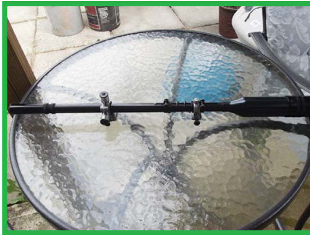
Top Left: The Davis Spot Shot scope was very long. About 30 inches overall. Top Right: The scope used Unertl micrometer mounts. Note the scope is moved to align the target. Not the cross hairs. Bottom Right: It's clear in this picture the vertical wire has broken away from the screw holding it in place. (Author Photos)
