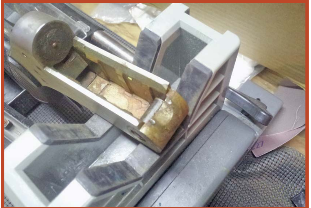
Left Photo: This is the underside of a shotgun forearm which has been neglected and rust has built up around the forearm attachment lug. Right Photo: Same single shot shotgun receiver where the rust has started on the inside of the receiver and around the firing pin on the bolt face. Looks like this may have been neglected for a few years. (Author Photos)
