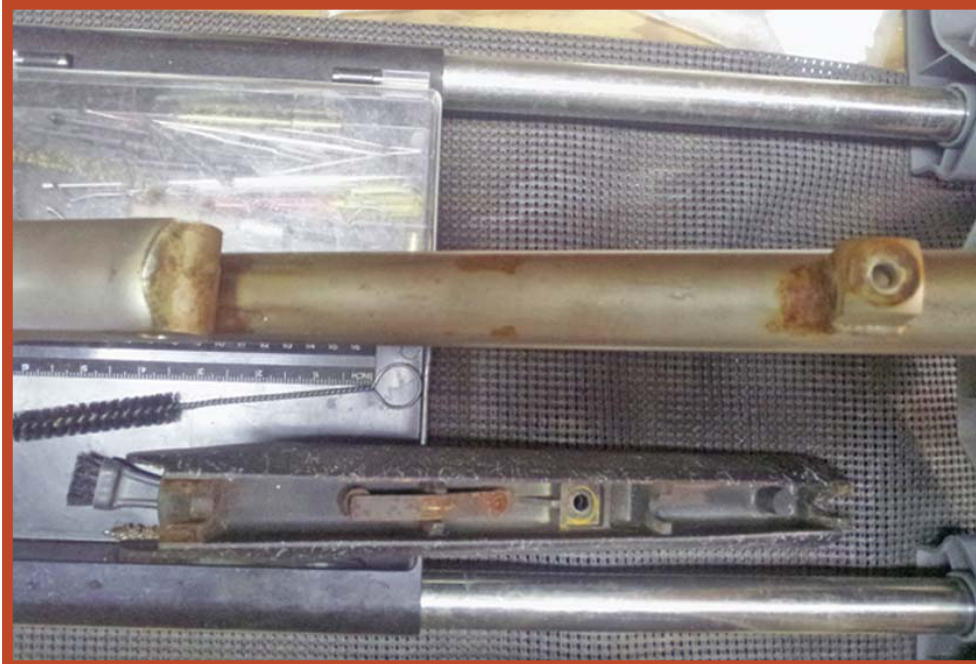
Left Photo: This is the underside of a shotgun forearm which has been neglected and rust has built up around the forearm attachment lug. Right Photo: Same single shot shotgun receiver where the rust has started on the inside of the receiver and around the firing pin on the bolt face. Looks like this may have been neglected for a few years. (Author Photos)
