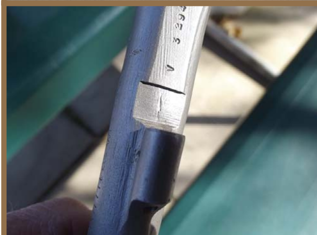
Top Left Photo: The Victory model as it was first brought to me. It had been partially disassembled. Top Right Photo: This view looking down the barrel from the muzzle. Notice the dark spot on the left side of the barrel about half way down the barrel. Middle Left Photo: This is the crack directly below the bulge in the barrel. The barrel could easily rupture with a standard .38 Special load, very likely with a +P load. Middle Right Photo: This is the finished product. New barrel installed, new Cerakote finish, assembled and tuned. The Cerakote finish is tough, good looking, and tough. Bottom Right Photo: The grip medallion shown is the reverse side of a Philippine coin. Possibly a ten, twenty, or fifty centavos piece. The date 1944 also agrees with when the gun was produced and may have been issued to a soldier in the Philippines. (Author Photos)
