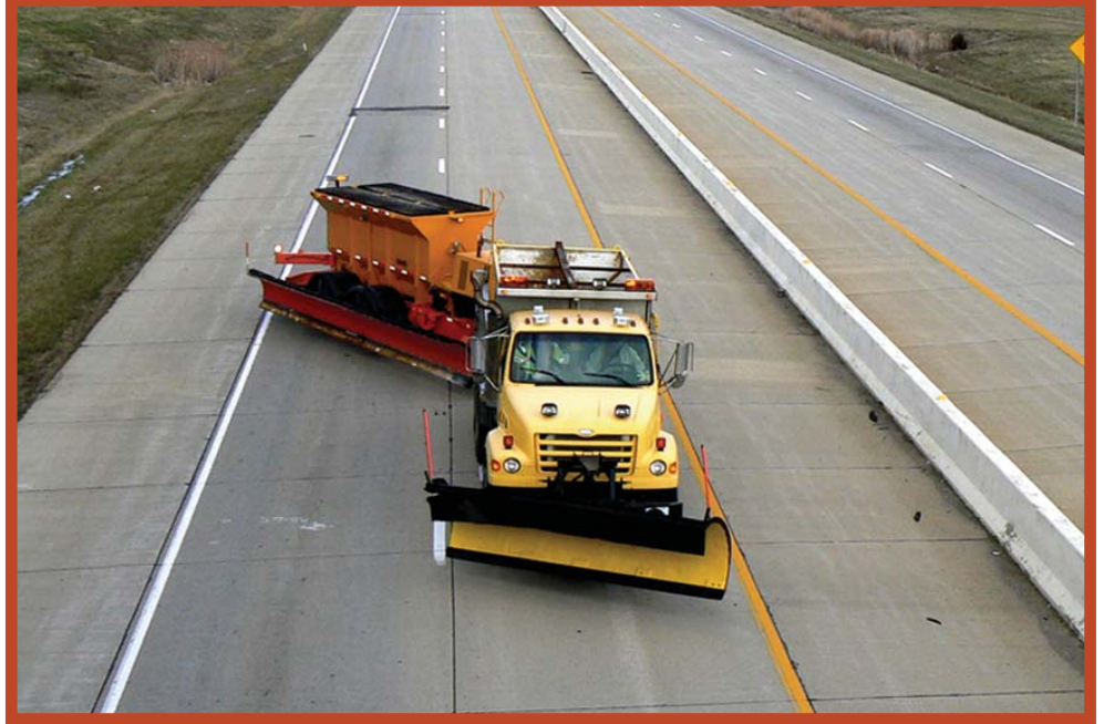
One of the new "Tow Plows" that allows INDOT to clear two lanes on a highway at once. Stay a safe distance behind when both lanes are blocked. (INDOT Photo)
