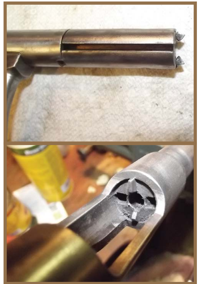
Photo 1: "Top extractor is new and fits a Browning Hi-Power and is the replacement for the lower extractor which the hook has broken off. Probable cause of breakage was dirt in the extractor slot." Photo 2: "When cleaning the bolt pay attention to the extractors and clean underneath the hook. The extractors should pitch in to pinch the base of the cartridge. If they don't, check to make sure there is no dirt in the extractor slot of the bolt. That may require removing the extractor from the bolt." Photo 3: "Clean around the slot and spring. Use your finger to move the extractor outward to make sure that it operates without sticking. Lightly oil the extractor spring (one half drop will do). If it is dirty or sticking you will need to remove the extractor, its spring, and plunger to clean the spring channel and extractor slot." Photo 4: "Note the extractor slots on either side of the chamber. Clean any debris from these slots and around the chamber. Clean the chamber of all bits of metal or dirt. To assure the chamber is in good condition look at the brass case of a fired round. Any bulges, scratches, dings on the case may indicate a problem in the chamber." (Author Photos)
