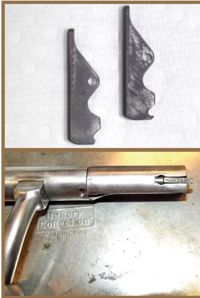
Photo 1: "Top extractor is new and fits a Browning Hi-Power and is the replacement for the lower extractor which the hook has broken off. Probable cause of breakage was dirt in the extractor slot." Photo 2: "When cleaning the bolt pay attention to the extractors and clean underneath the hook. The extractors should pitch in to pinch the base of the cartridge. If they don't, check to make sure there is no dirt in the extractor slot of the bolt. That may require removing the extractor from the bolt." Photo 3: "Clean around the slot and spring. Use your finger to move the extractor outward to make sure that it operates without sticking. Lightly oil the extractor spring (one half drop will do). If it is dirty or sticking you will need to remove the extractor, its spring, and plunger to clean the spring channel and extractor slot." Photo 4: "Note the extractor slots on either side of the chamber. Clean any debris from these slots and around the chamber. Clean the chamber of all bits of metal or dirt. To assure the chamber is in good condition look at the brass case of a fired round. Any bulges, scratches, dings on the case may indicate a problem in the chamber." (Author Photos)
