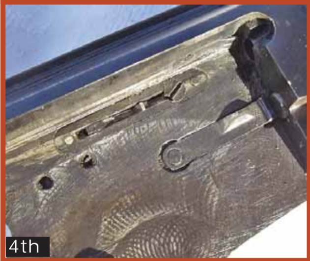
1st Photo: This is the Finger lever spring screw. There is no need to remove this screw. 2nd Photo: Firing pin on bottom is brass tipped and badly made. Firing pin on top is the correct firing pin. 3rd Photo: The ejector in its normal unlocked position. Note that the lock screw is aligned with the ejector. 4th Photo: The ejector in its locked down position for cleaning the bore from the breech. Note that the lock screw slot is not aligned with the ejector. (Author Photos)
