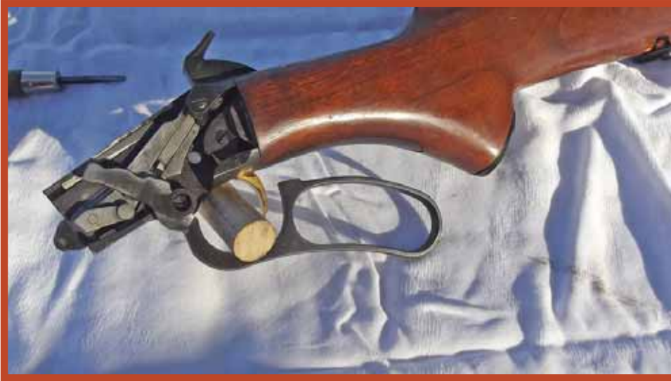
Left Photo: Here the Finger lever is not fully closed causing a dangerous situation. Right Photo: The Finger lever in the correct closed position and holding the bolt fully closed. (Author Photos)
