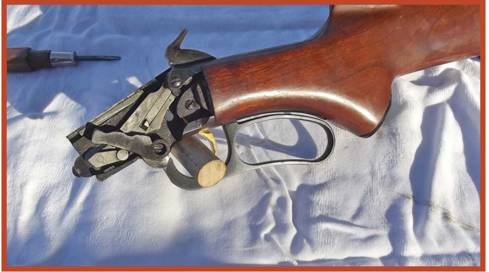
Left Photo: Here the Finger lever is not fully closed causing a dangerous situation. Right Photo: The Finger lever in the correct closed position and holding the bolt fully closed. (Author Photos)
