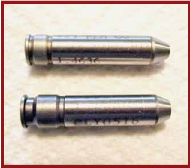
These are .223 Rem/5.56 Nato chamber gauges. The top one is the GO gauge and bottom is the NO GO gauge. I don't have or own any FIELD gauges. If the gun closes on the NO GO gauge I use a small piece of Plastigauge green or red to measure the additional headspace. (Author Photo)
