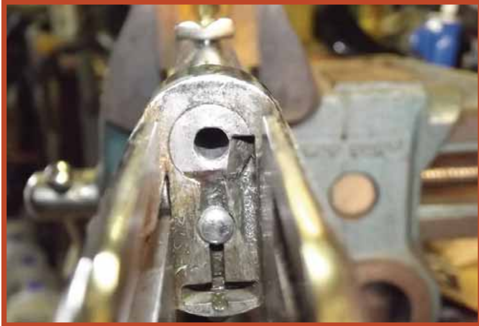
Left Photo: This is a view of the chamber on a 1906 Winchester .22 short. This one is in good condition for its age and years of use. Rust has pitted the barrel face but the chamber had not suffered any pitting. The chamber still required reaming with a special tool as the mouth had some denting from the firing pin been released on an empty chamber. It's safe to shoot. Right Photo: This is the chamber on a Stevens Crack Shot - 26. If you see a chamber in this good of condition it's a keeper as long as the rifling is not damaged. It wasn't. (Author Photos)
