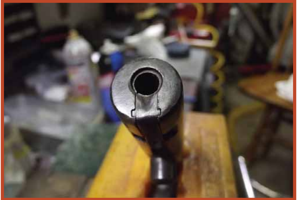
Left Photo: This is a view of the chamber on a 1906 Winchester .22 short. This one is in good condition for its age and years of use. Rust has pitted the barrel face but the chamber had not suffered any pitting. The chamber still required reaming with a special tool as the mouth had some denting from the firing pin been released on an empty chamber. It's safe to shoot. Right Photo: This is the chamber on a Stevens Crack Shot - 26. If you see a chamber in this good of condition it's a keeper as long as the rifling is not damaged. It wasn't. (Author Photos)
