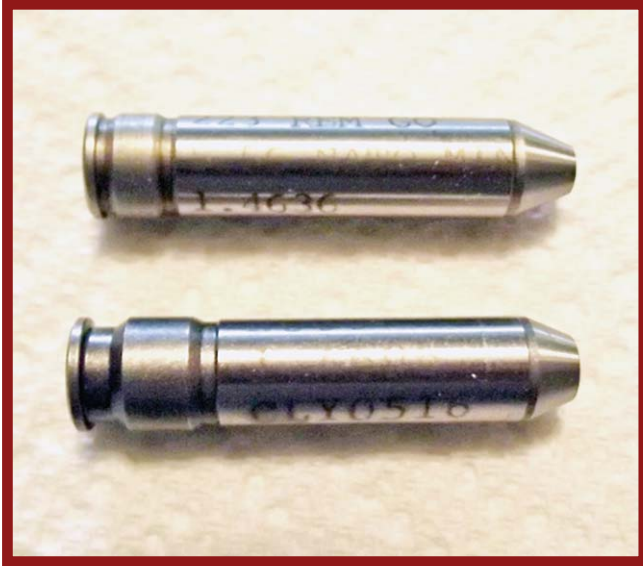
These are .223 Rem/5.56 Nato chamber gauges. The top one is the GO gauge and bottom is the NO GO gauge. I don't have or own any FIELD gauges. If the gun closes on the NO GO gauge I use a small piece of Plastigauge green or red to measure the additional headspace. (Author Photo)
