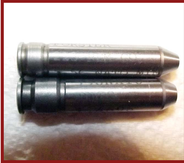
Again I apologize for the poor photography. I'm attempting to show the difference in the 2 gauges. The NO GO gauge is .006" longer than the GO gauge. Maximum SAAMI headspace dimensions is .010" over the minimum which the GO gauge measures. The gunsmith will try chamber the gun so that the GO gauge just fits. (Author Photo)
