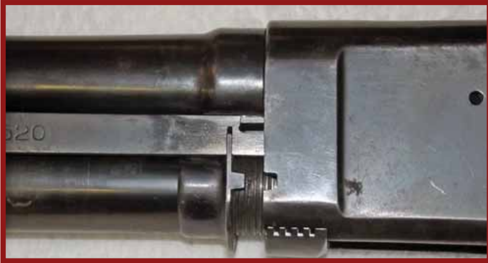
Left Photo: Showing the magazine nut backed out from the receiver. Move the barrel assembly down about 1/4" and push the action slide forward so the action bar is clear of the receiver. Right Photo: Separate the barrel assembly and receiver and set the barrel aside. (Author Photos)
