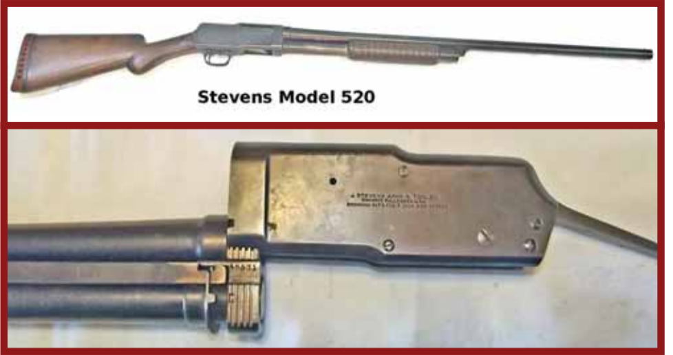
Left Photo: Showing the magazine nut backed out from the receiver. Move the barrel assembly down about 1/4" and push the action slide forward so the action bar is clear of the receiver. Right Photo: Separate the barrel assembly and receiver and set the barrel aside. (Author Photos)
