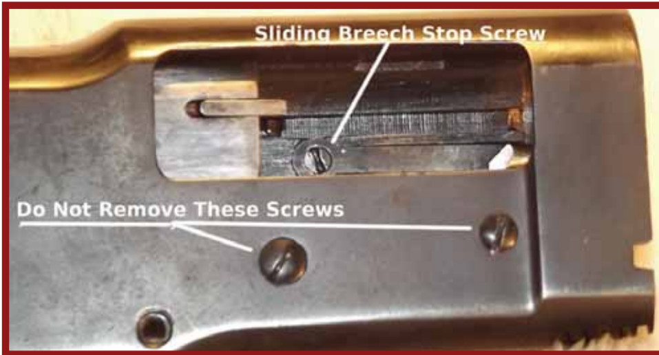
Left Photo: Right Receiver, remove the screw in front of the bolt in the picture to remove the Sliding Breech Stop. The screw heads shown as Do Not Remove are staked in and should not be removed. Right Photo: See body of article for description of parts. (Author Photos)
