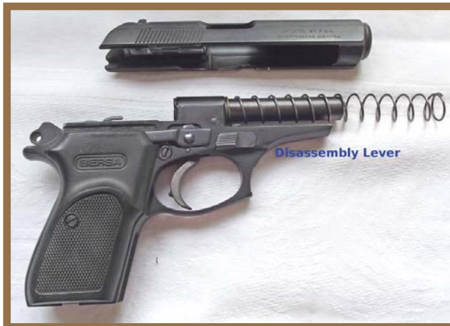
The Bersa Thunder 380 field stripped. Easy to disassemble and clean." (Author Photo)
